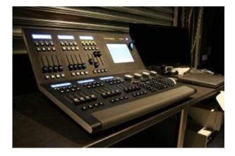
Johnny explains, "To do this we had to include a Strand DMX Merge Controller, so that the operator could merge the Philips Strand 500ML desk which would take over the control when they have events other than the cinema."
