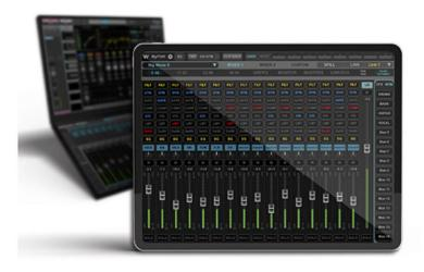
Waves MyFOH is a remote control app for the Waves eMotion LV1 Live Mixer that allows front-of-house engineers to control the LV1 over WiFi, from any iPad or Android tablet, and shape the live mix from anywhere in the venue.
