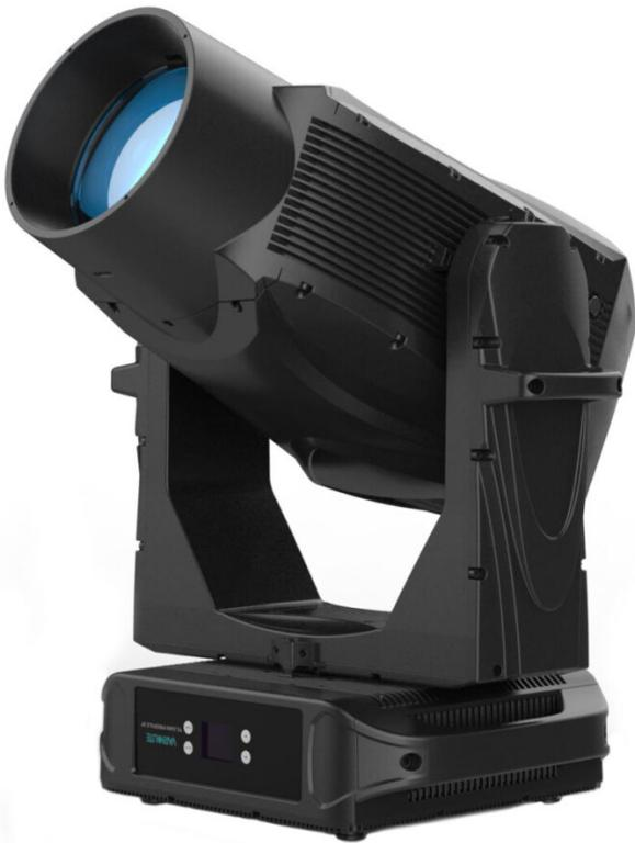
With a 1000W monochromatic light engine producing 85,000 source lumens, the VL3600's huge output power is ready to light the show from any distance in any weather. Thanks to a CMY+CTO color wheel mixing system, the fixture produces a wide range of rich colors while eliminating the appearance of blades in the lens, improving direct view applications. With dedicated CRI boost and color correction filters, colors render beautifully on stage or on camera.
