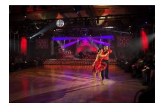
A box truss was flown over the low ceilinged dancefloor, approximately 14 metres long by 10 metres wide, giving about 4 metres of headroom, and this was interlaced with 4 trussing ribs traversing the width of the space.
