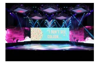
The Robe ColorWash 2500s were primarily used for camera work as the shows were filmed for Comedy Central. Gobo effects on the stage floor were created by the Robe ColorSpot 2500. Sean used the Robin 600 LEDWAsh to add colour and compliment the video material.
