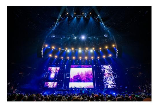
The back truss was rigged with 12 x FORTES, picked for their intense power and impact to project textures on the red velour drape behind the video wall, with another 13 x FORTES on the front truss, working with four more on the advance truss. These last four FORTES were all running on a 4-way RoboSpot system.
