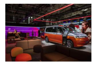
Four Robe RoboSpot remote follow spotting systems, controlling four of the FORTEs, were specified for the flurry of events and presentations during the expo's press day, and there were also 58 x Robe LEDWash 800 luminaires fitted with beam shapers and top hats dotted around specific areas of the stand highlighting cars and the pop-up press area / broadcast studio.
