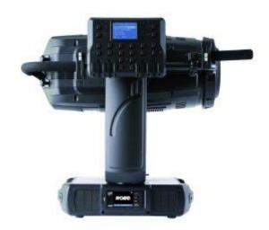
BMFL LightMaster is an accessory comprising externally mounted, fully programmable follow-spot handles with a control panel and two individual faders that enable any of Robe's BMFL range of fixtures to be run as a follow spot.
