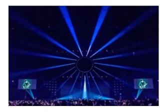
There are 8 overhead trusses including a distinctive 20ft diameter circular truss flown directly above Mendes' central marks – dubbed the 'halo' by the creative team. Two of the trusses are upstage of the screen for blow-through lighting effects and another two 'wing' trusses extend the stage sideways into the arena.
