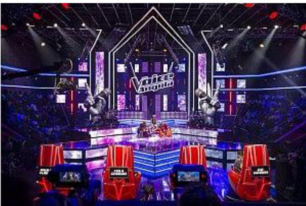
Josh also wanted a lighting ‘backdrop’ at the stage end that could be pixel mapped, so a grid arrangement includes 12 x Robe CycFX 8s and 24 x LEDBeam 100s together with LED panels and battens.
