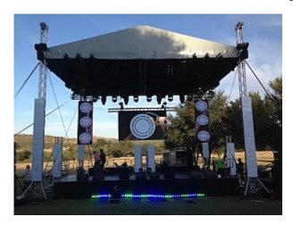
Showgroup were the technical supplier and incorporated a Prolyte Roof Structure used for the stage, 16 Robe Robin 300s and 4 Robe BMLFs. Other lighting included 6 Martin Mac 600s, 30 x Stage Color 48, 24 Longman LED Cans, 20 x Longman Colourme 11, stage battens, 12 Parcans and 6 x Source 4 Profiles
