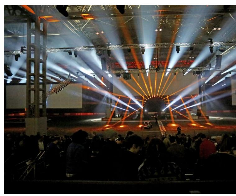
A network of trusses was rigged in the roof, trimmed at 9 metres, including four 90 metre long sections, one above the audience and three 'stage' left and right over the track and another two 20 metre long side trusses, all
