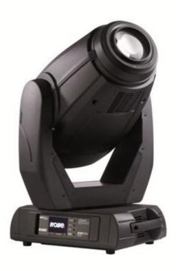
This is an amazingly bright 1200-series equivalent lightsource utilising Robe's popular MMX optical technology, complete with a framing shutter system comprising four fast 'blades' that can be individually positioned and angled plus or minus 45 degrees, with the whole Blade module capable of plus / minus 90 degree rotation.
