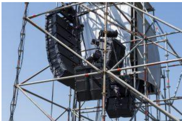
Main tower systems comprised eight inward facing hangs of six K2 with four KS28 subs with fill speakers of three hangs of 11 Kara each. Photo credit: Martin Reid.
