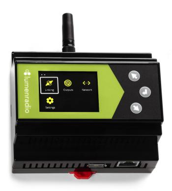
Galileo MAX is LumenRadio's latest addition to the Galileo family of Wireless DMX products used primarily for architectural lighting.
