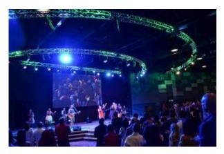
DWR Distribution were honoured to be commissioned to install a lighting solution which had to be ready for the official opening held in January 2017. Control is via MA on PC Command Wing. The moving lights comprise of Robin Spiiders and Robin miniPointes, while Philips Selecon SPX Axial 19 Degree and various LED Pars are used for generic lighting and truss warmers.
