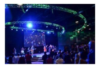
DWR Distribution were honoured to be commissioned to install a lighting solution which had to be ready for the official opening held in January 2017. Control is via MA on PC Command Wing. The moving lights comprise of Robin Spiiders and Robin miniPointes, while Philips Selecon SPX Axial 19 Degree and various LED Pars are used for generic lighting and truss warmers.
