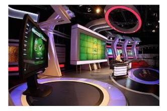
Additionally, 1.3km of LED strips were used, both in the studio and in the refurbished studio garden; these were used to display team colours of the duelling teams on any given match. However, this proved to be one of the challenges for DWR's team under Bruce Riley as each strip had to be on an individual, dedicated circuit to differentiate their identities.
