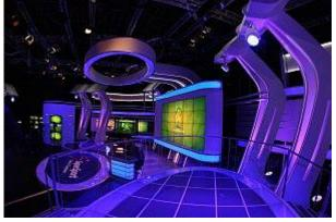
"With the technology of LED fixtures for camera," says Cutts, "the light spills everywhere and as much as that spill can sometimes be negative, if you use it positively it can spill and wash your set and your audience very quickly and easily. With white Tungsten light things become flat very quickly. The challenge was to keep the lighting contained in all the areas."
