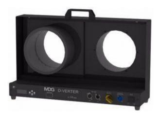
Unique to MDG, D-Verter 239 is a DMX/RDM pneumatic 23 cm (9―) input/output fog switcher designed mainly for use with ICE FOG Q. It performs several functions by using a sliding conduit either to split a single source of fog into two distinct outputs, merge two separate sources of fog into a single output, or act as a fog output gate.
