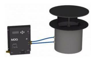
RFP 239 is a DMX/RDM-operated pneumatic Round Floor Pocket of rugged construction which can be embedded in the stage floor or set wall to conceal a fog output. It is intended to operate under pneumatic pressure as part of an existing fog system, delivering low fog or fog to precise locations.
