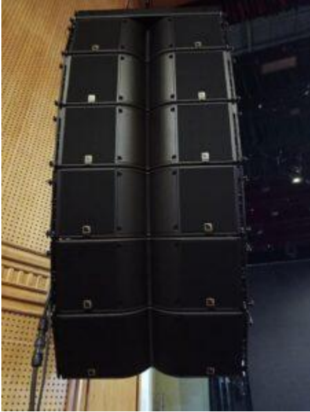
Six L-Acoustics K3 per side rigged up
