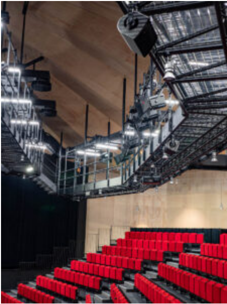
L-Acoustics X8 are mounted on the truss for delay in The Galabru theatre.
