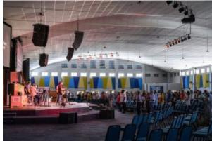
The lighting request was straightforward. The church already had some Longman fixtures used as stage washes. DWR added two lighting bars to the church's existing bar and supplied a further 12 Longman F8UP (45 degree), four Longman F4UP (25 degree) and new cabling infrastructure.
