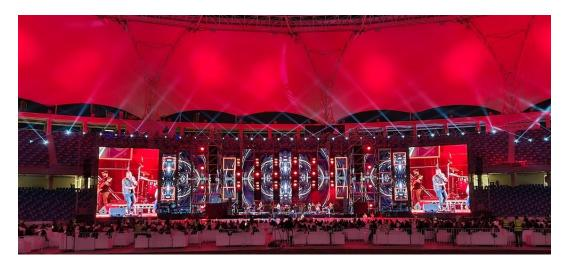
The final setup comprised main hangs of 12 K2 atop six Kara per side, with 12 stacks of two Kara atop two SB28 subs, evenly spaced in front of the stage lip. A further 60 Kara, 12 SB28 and eight SB18 catered for delays, while stage monitoring comprised two stacks of six Kara atop four SB28 for sidefill, plus 24 X15 HiQ along the stage lip. Control was via a total of eight LA12X and 27 LA8 amplified controllers.
