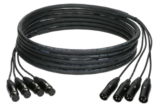
The excellent layer stranding of the elements to the cable core maintains their structure even under high loads and an aluminium-coated foil (PiMF) effectively protects the individual pairs from electromagnetic interference. The black PVC outer jacket is very robust and yet offers pleasant flexibility.
