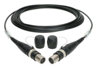
A highly flexible construction with 500 ?m primary coating and 900  $\mu$ m tight buffered fibre construction reliably protects the fibres (4 x 9/125  $\mu$ m, OS2, 4 x 50/125  $\mu$ m, OM3/4) from external influences and allows even the smallest bending radiuses with a cable diameter of just 6 mm.
