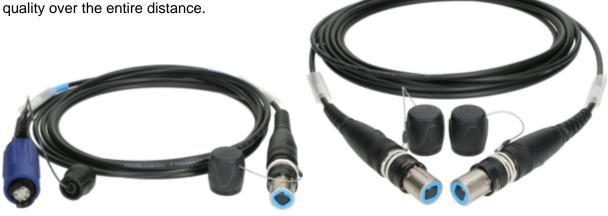
The robust metal housing of the opticalCON® QUAD cable connector conceals a connector with four optical multi- or single-mode PC resp. single-mode APC channels, based on the renowned LC technology. When plugged in, the optical fibres are in physical contact. The automatically closing protective flap with silicone seal provides dirt and water tightness according to protection class IP65. Additional practical features are the proven push-pull locking and a very efficient strain relief.
