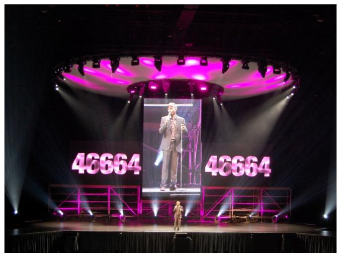
The screen was made up from Lighthouse Technologies R16i/o ll modules. The top was 69 metres high and the sides 14 metres wide and it was supplied by LED Vision. LEDVision's Operations Manager Allen Evans managed the LED aspects onsite as well as camera direction.
