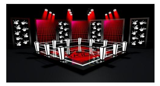
For *The Voice Kids*, Fuentes and his team positioned LED screens on every wall of the set. All were different sizes, including tall strips of 1m x 4.5m to contrast others at 3m x 4.5m. Between these screens, 3m x 4m boxes with the *The Voice* logo were displayed, illuminated by LED nodes mapped and controlled by the programmer. On the main stage floor, they placed LED strips of 6m x 0.5m right in front of every TV judge featured on the show.
