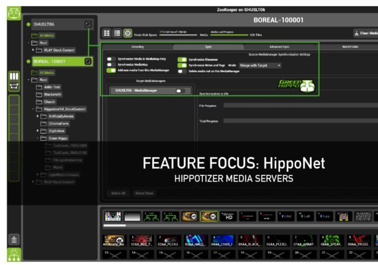
The heart of Hippotizer<sup>™</sup> is HippoNet, the networking protocol which connects all Hippotizer machines together so that one ZooKeeper can control all the networked systems at once. HippoNet distributes timecode, media and playback synchronisation between systems to effortlessly control even the largest systems.
