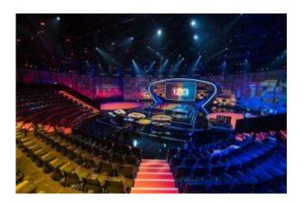
The live event itself saw mo2 design use four Hippotizer Boreals – teamed with a pair of grandMA2 lighting desks – controlling four Barco HD 30.000 projectors creating a four-cube wall, a further two Barco HD 30.000 projectors enabling rear projection, plus an LEDGO Black Spinel LED floor.
