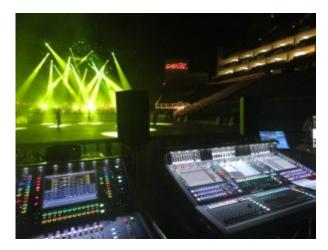
"With this sort of sized show, we have to be on top of things," Butcher explains. "Dave writes the spec, and we all add to it. Rack-wise, we have three SD racks and one [DiGiCo] Orange Box, and that's got two MADI outs – it is the digital in for the keys and tracks, and sends for record. So we're patched for that as well.
