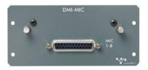
The S-Series has already benefitted from an increase from 40 to 48 flexi channels as part of a recent update, and the new DMI-MIC Pre-Amp Card adds an extra eight mic inputs, connected via a 25-way D-sub, using the same great pre-amps already found in the console. This allows for up to 40 mic inputs directly on the console surface.
