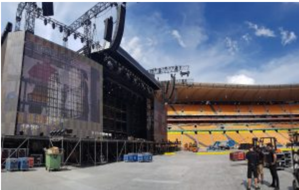
Main hangs of K1 and SB28, along with K1 delays delivered improved coverage for this yearâ€™s festival.
