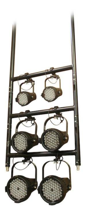
Faster rigging of stage and sets combined with improved safety are just two of the benefits offered by Doughty Engineering's Modular Rigging System. A strong, safe alternative to 'home made' drop arms, which until now have been the only option for riggers, the system uses tried and tested connectors to give a SWL of 100kg and enables the safe and speedy rigging of luminaires from truss or fixed tubes or barrels. It also provides for a
