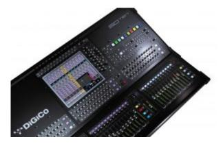
L-ISA Source Control for L-Acoustics L-ISA immersive technology has been natively integrated into SD-Series, adding L-ISA's object-based mixing technology to the console's control surface.
