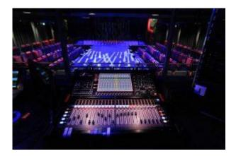
The SD9 and a DiGiCo Orange Box are key to the system – which includes an extensive EM Acoustics loudspeaker system, QSC digital signal processing and Sennheiser microphones – with system inputs being fed through it as required. It is programmed as an LCR and Sub system via the matrix outputs, with the provision for more inputs if needed.
