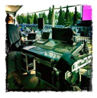
House consoles for the main stage were a DiGiCo SD10 and SD12 for front of house and an SD10 at the monitor position, plus an SD-Rack with 32-bit Stadius I/O cards. Guest consoles also included an SD9 and SD5.
