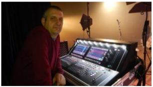
Mark has owned his S21 since last year and has added a SoundGrid card, with a DMI MADI B card handling the inputs from the D2 Stage Rack.
