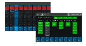
The release of V2.6 also sees the addition of an RTA (Real Time Analyser) added to the channel EQ view of S Series consoles, which can be toggled to be shown/hidden using the button in the top bar. The RTA meters are taken post-EQ, meaning that any adjustments in EQ are reflected in the RTA's metering.
