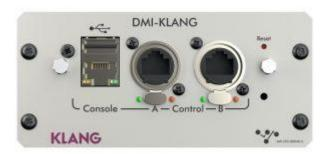
The DMI-KLANG takes KLANG:fabrik's immersive in-ear mixing core and rebuilds with today's latest FPGA technology to deliver immersive mixes of 64 inputs for 16 musicians. This is the highest input count of any KLANG product to date, with a processing latency of just a quarter of a millisecond. The DMI-KLANG connects directly to DiGiCo consoles' internal audio stream without any additional hardware I/O overhead.
