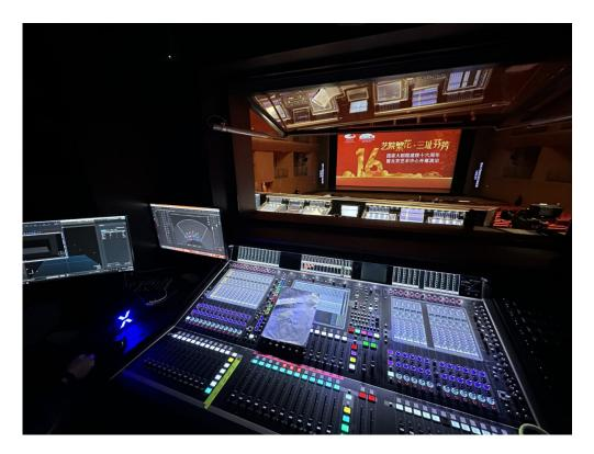
Two mirrored Quantum 7s backstage and two mirrored SD5s at the front of house position were connected via an optical network, providing the interfaces that engineers Wang Bin and Wang Lei needed to ensure the different styles of performance were able to sit together in Wang Bin's immersive mix.
