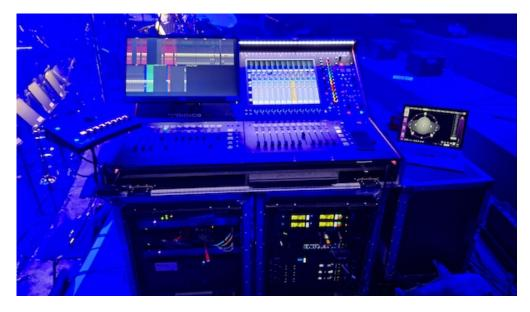
Manoeuvrability was a major part of the Quantum 338's attraction for Wright, weighing in at 70kg, it is over 40kg lighter than the larger Quantum 7 series consoles but still packs a weighty punch in terms of onboard processing.
