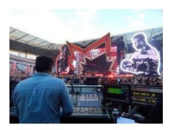
"Around 96 inputs come from the stage, plus a large amount of inputs for band talkback and comms, which allow the band to communicate with the techs and Jonathan at monitors," says Josh. "On top of this, we have triggers on the drums just to key the Gates on the console. Before you know it, the racks are all full!"
