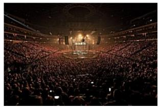
Using WYSIWYG, Havli?ek designed and coordinated the production's large-scale light show. The design centralised around a central 360° drop of four concentric circular trusses on Cyberhoist motors. LED screens faced each truss to partially mask the mix of Claypaky Sharpy, Claypaky A.LEDA K10 and Claypaky Alpha Spot 1200 that provided the lighting from the show's centralised column.
