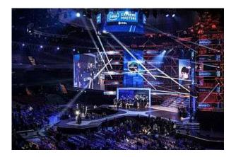
The multimedia equipment consisted primarily of two huge 17 x 9 yard screens and two interconnected Barco projectors, which were used to project images with an overall brightness of almost 50000 ANSI lumens. A total of nearly 240 square yards of Fourlight LED Grids, Curve 8s, Flex LEDs and LED screens were used on the main stage. Moreover, the horizontal lines on the stairs and in the central part of the video strips were made using over 328 yards of Hi-Strip.
