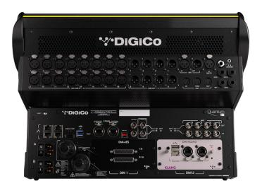
Other highlights include Stadius 32-bit ADC and DAC conversion, dual DMI slots, and a host of versatile I/O options, including Dante (64 channels in and 64 channels out at both 48kHz and 96kHz), MADI (redundant or single), optional optics, AES, local connections (16 analog inputs and eight outputs), and more.
