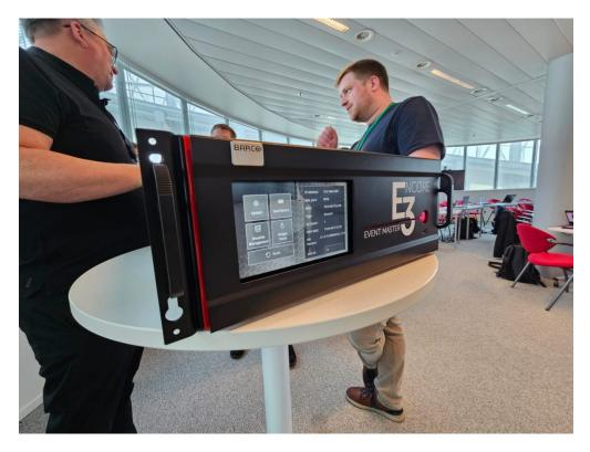
Barco Encore 3 is a state of the art video processor that delivers exceptional native 4K image quality with best-in-class Athena scaling and ultra-low processing latency down to 16ms. The Encore 3 provides access to a boundless canvas at 12-bit 4:4:4 processing with no fewer than 16 fully capable 4K60 layers per screen.
