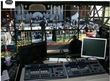
Brisbane Concert Lighting was again the main equipment supplier, supplying all control from LSC Lighting Systems, including Clarity (using 6 DMX universes) with two VX20 wings, five e24 Dimming Systems, five Delta Power Distros and three Delta DMX splitters. The LSC control equipment looked after 44 Martin Moving Lights, 32 LED Par 64s, 32 LED strips and over 72 Fresnels, Pars and Profiles.
