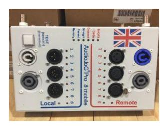
DWR Distribution is delighted to supply CableJoG to the South African market. Based in the United Kingdom, CableJoG design, manufacture and distribute a range of cable testers from 12 test points in the case of the AudioJoG Pro audio cable tester and AudioJoG Rack through to 1024 in the CableJoG 512 cable tester with the extra 512 adaptor.
