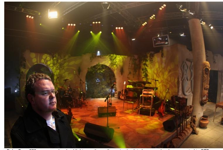
Robe Scan 575s were used as backlight over the audience to simulate beam work colour corrected to CTB, into the camera. The units were rigged on trussing above the audience.
