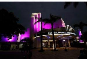
The Durban area has a very corrosive environment with high humidity, salt in the air and spectacular coastal thunder storms, which is why they reverted to using neon instead of LED strip lights as the outliners. "We are quite certain that plastics may corrode and become brittle due to the amount of atmospheric UV" says Joao.
