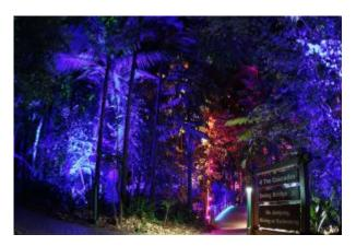
The water features – there are two, one each side at the start of the pathway – which were previously in total darkness – are now energised with colour and movement with the help of 12 x ArcSource 24MC Submersibles. These skim the surface of the water with light, and units are also fixed in place directly below the fountains and focussed upwards, changing the look and feel of the dancing water jets.
