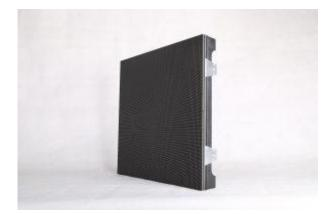
Visitors to Mediatech Africa will see the bright Polaris Lite 3.9mm indoor screen as they enter the exhibition area. The advanced auto-lock and auto-eject system, allows panels to be attached together by magnets. An inner and outer curve lock system maintains the highest level of alignment accuracy in both flat or curve configuration. Panels are lightweight, weighing 9kg per panel.
